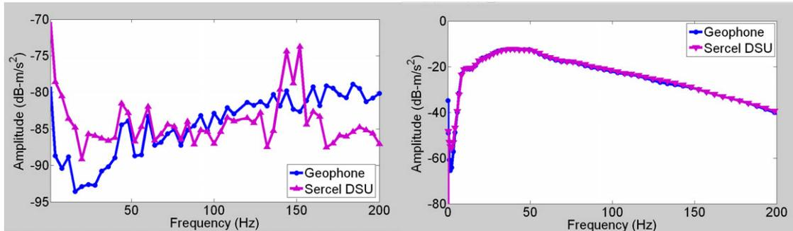
Figure 4. Acceleration amplitude spectra. Left: Noise before first breaks. Right: Average of all traces (0-4 sec).
