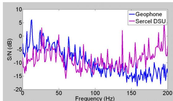
Figure 5. Acceleration domain spectra, noise before first breaks.
