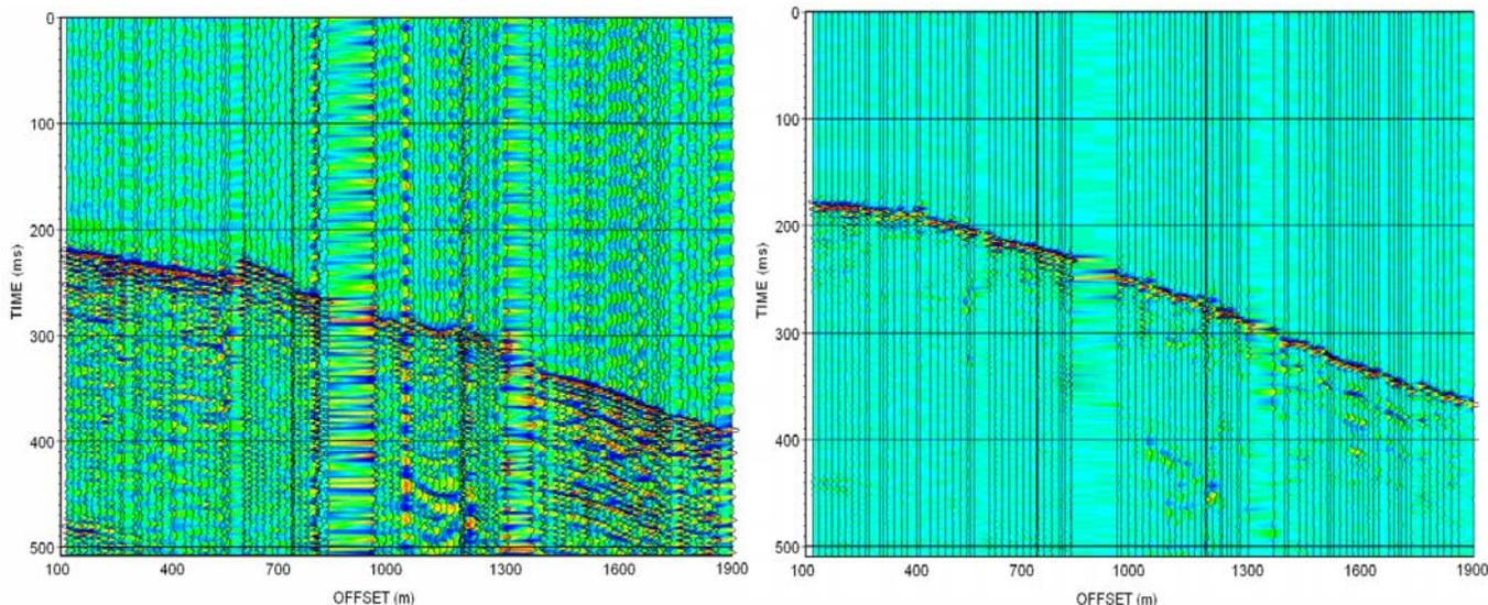
Figure 2: Seismic traces of the Northeastern 1000 m walk-away VSP, in the time-offset domain, before (left) and after static corrections and filtering to enhance the P-wave arrival (right).
