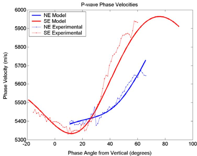
Figure 4: Experimental anisotropy results between 50-1000 m in depth along both azimuths, and the theoretical model results along the same azimuths.
