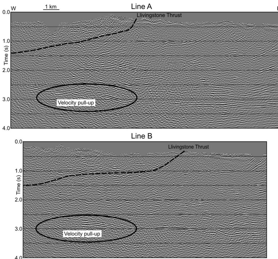
**Figure 1.** Post-stack time migrated sections. The Livingstone Thrust carries some high velocity carbonates in its hangingwall, which contribute to a velocity pull-up on the time sections.
