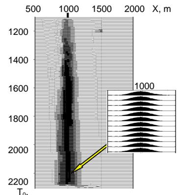
**Figure 5. Seismic image of side wall of the salt dome by Duplex Wave Migration.**
