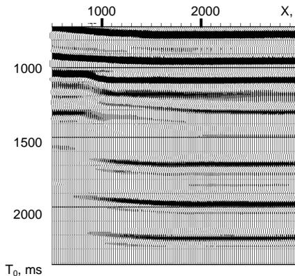
**Figure 4. Seismic image of cross-section by conventional CSP migration.**
