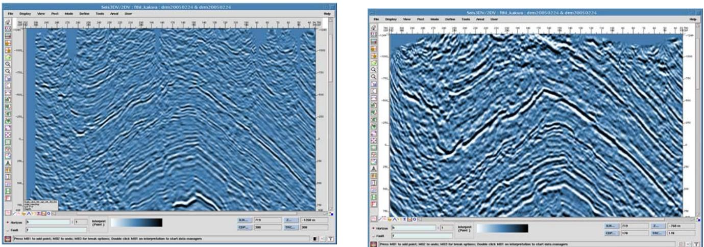
**Figure 3. Zoom of the upper part of the same dip line. Left: “Model Driven” Anisotropic PSDM, Right: “Data Driven” Isotropic PSDM. Note the Isotropic PSDM much more clearly resolves the structure and faults, which are barely present on the Anisotropic PSDM.**
